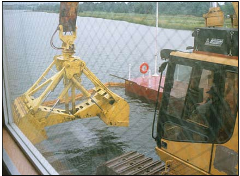
Mechanical dredges similar to this will be used in the first phase of dredging in the Upper Hudson River, scheduled to begin in 2009.
