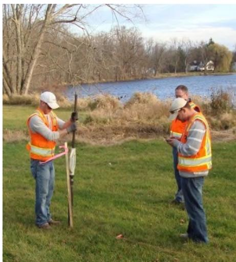
*Taking a soil sample is a simple and routine process. Samples are collected using hand tools (such as hand auger) and result in a 2-inch diameter hole. After each sample is taken, the hole is filled in. Because near surface soil generally represents the greatest potential risk to human health and the environment, samples will typically be taken to a depth of 1 foot. Some deeper samples may be collected.*
